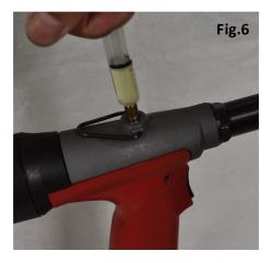
2. Fill the syringe (supplied with the tool) with hydraulic oil. Screw the filled syringe in the oil fill screw hole. Inject all of the oil in the syringe into the tool, adequate oil has been added if there is oil flowing back to the syringe when you loosen your hand, then keep pressing the syringe for two or three times, in order to prevent air go into the oil in the tool. (Fig.6)
